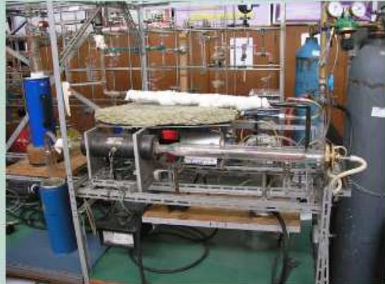
System for combustion of organic samples - obtaining of CO<sub>2</sub> for subsequent preparation of benzene
