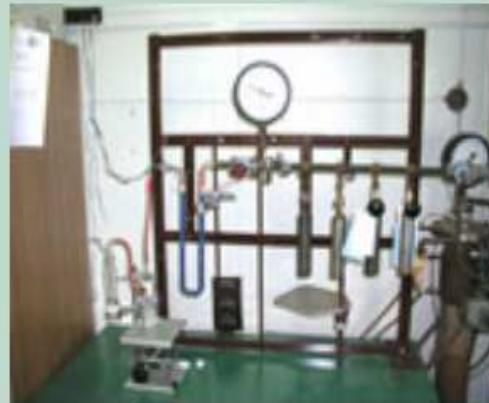
Vacuum line for direct absorption of CO<sub>2</sub> for <sup>14</sup>C activity measurements by LSC
