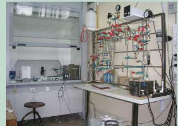
Vacuum line for benzene preparation for <sup>14</sup>C activity measurements by LSC
