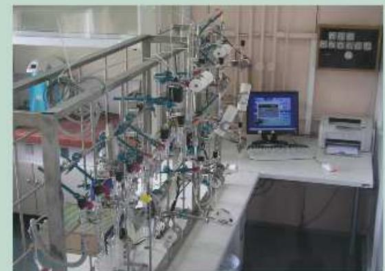
Vacuum line for preparation of graphite for <sup>14</sup>C AMS measurement technique
