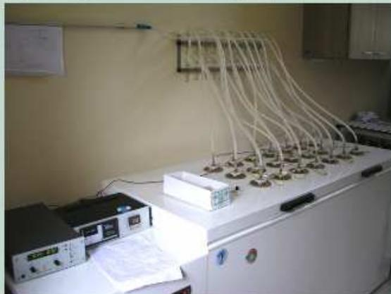
System for electrolytic enrichment of water with tritium for <sup>3</sup>H activity measurement by LSC
